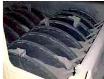
MultiDisc® Thermal Processor Used in the Chemical Industry
